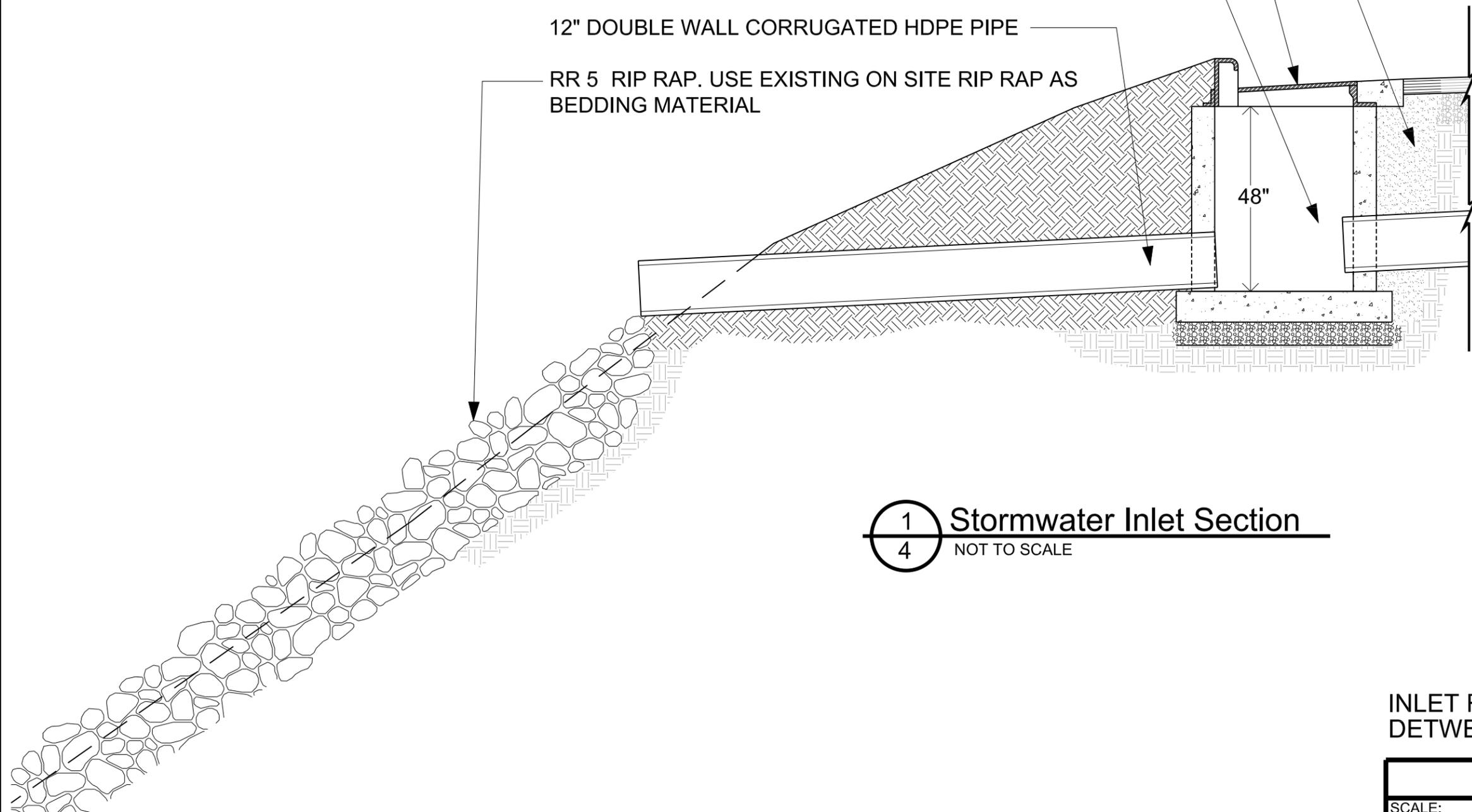
1 Stormwater Inlet Section
