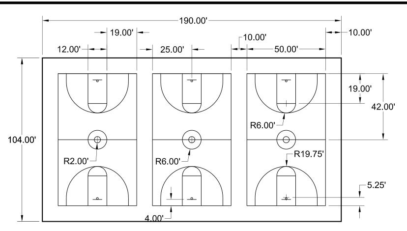
Existing basketball standards to remain. Remove all existing HMA courses. Blade and compact aggregate base course. Report any voids or discrepancies to the Owner's Representative. Place and compact 1-1/2" leveling course and 1-1/2" surface course HMA. Court lines shall be 2" width white lines. Verify striping dimensions with existing basketball goals to remain.
