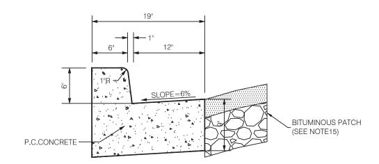
NOTE: CONTRACTION JOINTS ON THE PROPOSED CURB AND GUTTER SHALL BE MADE BY SAWING AT INTERVALS OF NOT MORE THAN 15 FEET. SAW CUT TO BE NOT LESS THAN 2" DEEP. NO DOWEL BARS REQUIRED.
