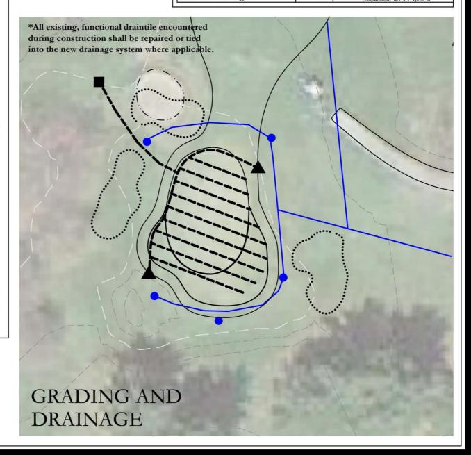
In existing green areas, sod shall be stripped over trench areas only (5"-6" wide), temporarily stockpiled, and replaced in same location following drainage install. Sod shall also be stripped and replaced in rough areas over top of outlet pipes.
