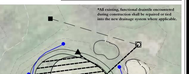
In existing green areas, sod shall be stripped over trench areas only (5"-6" wide), temporarily stockpiled, and replaced in same location following drainage install. Sod shall also be stripped and replaced in rough areas over top of outlet pipes.
