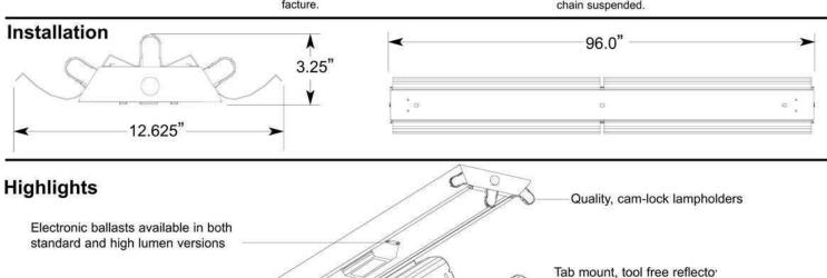
Computer designed, CNC formed 0.020" specular aluminum reflector
